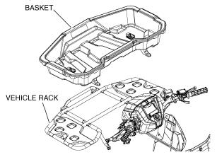
Secure the cargo box to the vehicle by pressing down each Honda Pro-Connect<sup>™</sup> latch lever.
